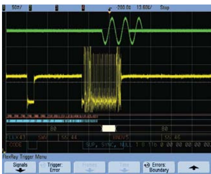
See mixed signal measurements in a FlexRay system using an MSO.
