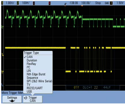
Trigger on and decode CAN serial packets.
