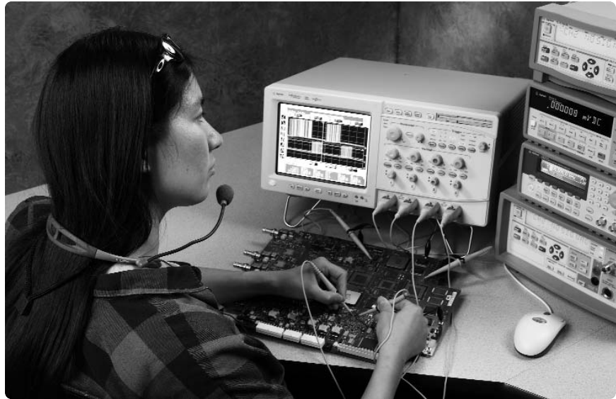
Figure 11.1. VoiceControl allows you to control the scope hands free.
