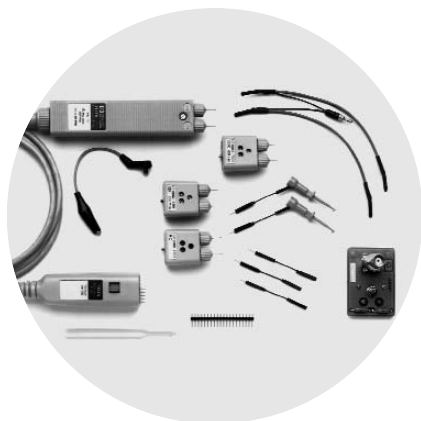
Figure 4.1. Agilent 1153A for probing low-bandwidth differential signals.
