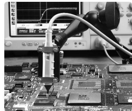
Figure 3.13. Agilent E2654A EZ-Probe Positioner option provides stable and accurate X,Y, Z probe positioning (see “EZ-Probe Positioner” in the “Probing Accessories” section of this document).
