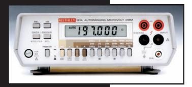
The Model 197A is a lightweight, portable DMM with a battery pack option. It combines 5½-digit resolution (on a 220,000-count display) with  $1\mu$ V, 1nA, 1m $\Omega$  sensitivity. Basic DCV accuracy is 0.011%.
