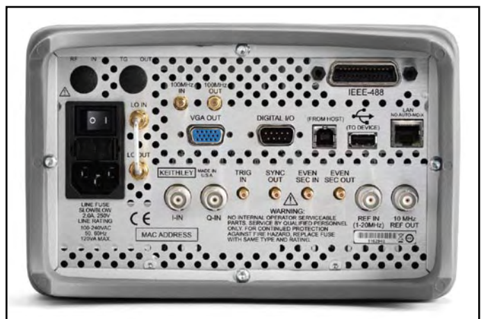
Model 2820 rear panel. Note the RF input (2820-R configuration option).
