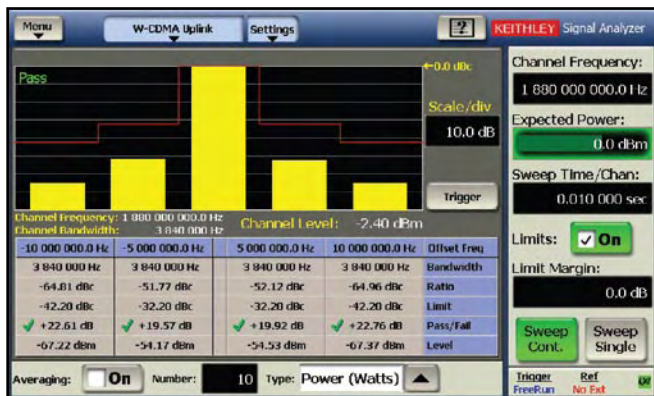
Use the Adjacent Channel Power Ratio function to define the test parameters and the test limits for non-standards-based signals.
