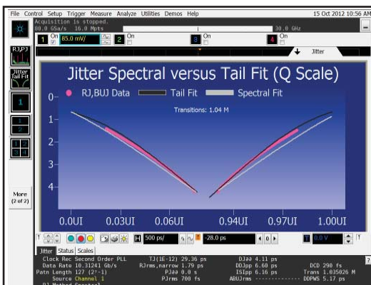
Jitter separation makes debugging your device easy
