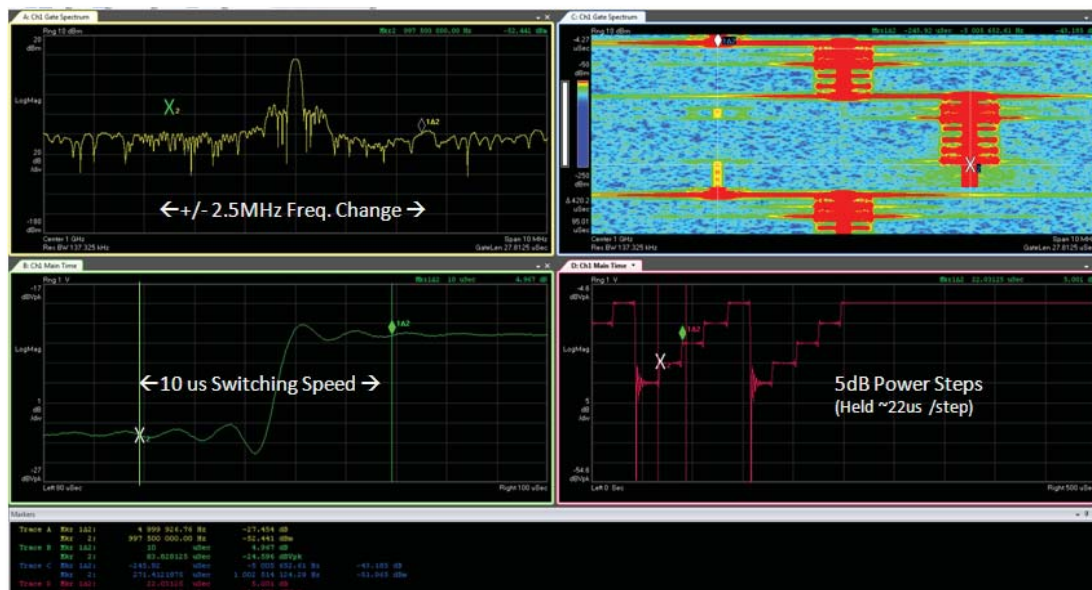
Figure 2. M9381A baseband power and frequency offset tuning in < 10 \mu s as shown by the 89600 VSA software.
