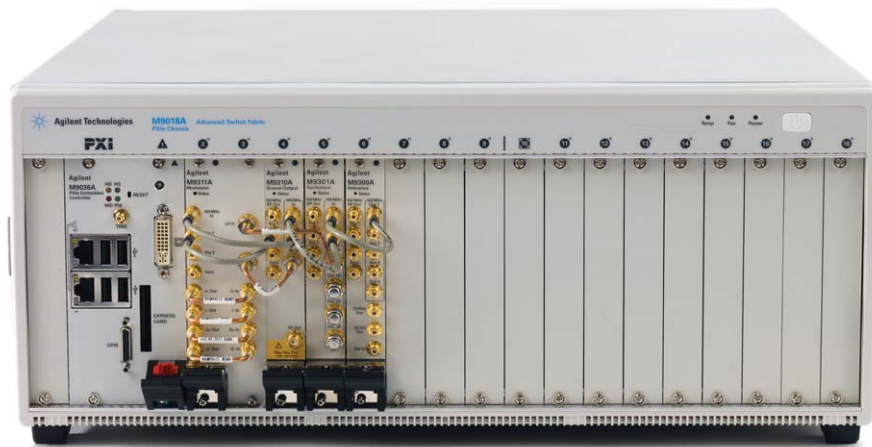
Figure 19. M9381A PXIe vector signal generator with four modules consisting of the M9311A digital vector modulator, M9310A source output, M9301A synthesizer and the M9300A frequency reference placed within the Agilent M9018A PXI chassis with the Agilent M9036A controller.
