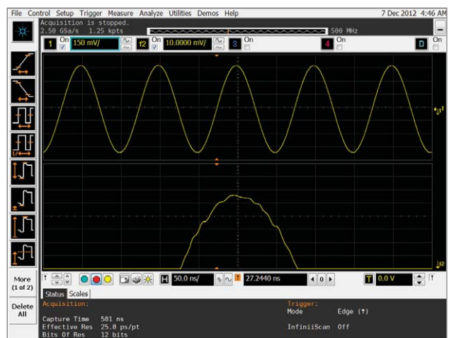
Zoom on top of same clean sin wave with equal bandwidth 9000 H-Series scope shows significantly less noise
