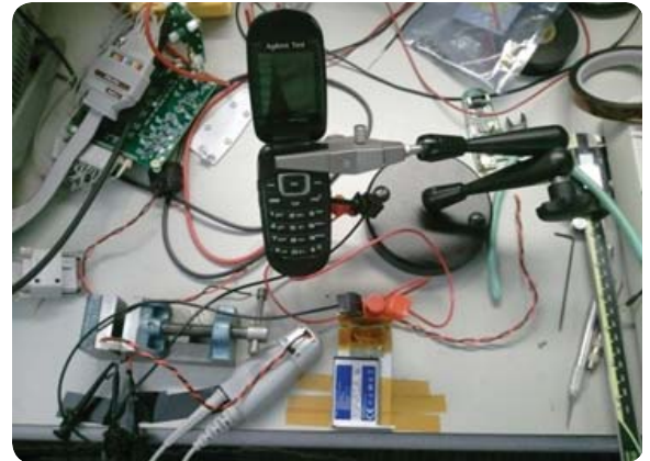
Agilent's ultrasensitive N2820A/N2821A current probes excel at measuring with resolution as low as 50 uA for small current levels typically found in mobile devices. Or, the probes can be configured for current up to 5A.
