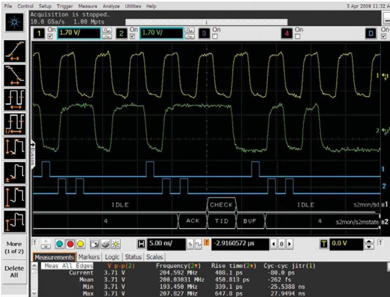
Use the MSO timing channels to evaluate control signal relationships and data buses up to 16 bits wide. Use symbols to more quickly interpret waveforms.
