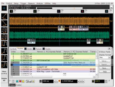
Trigger on and decode PCIe serial packets.
