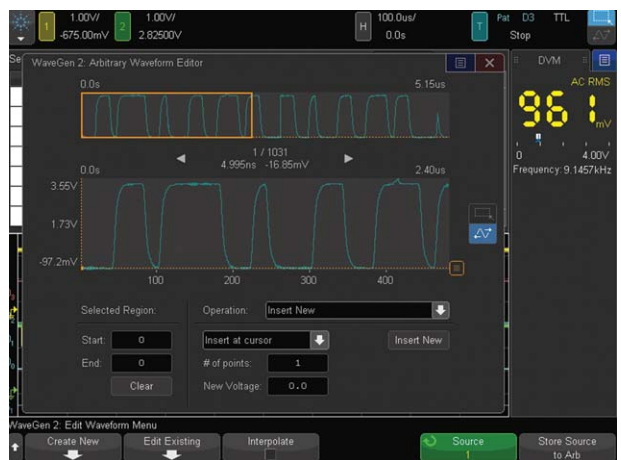
Figure 22: WaveGen arbitrary waveform editing screen.
