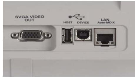
Figure 36: Standard VGA output, USB host and device and LAN.
