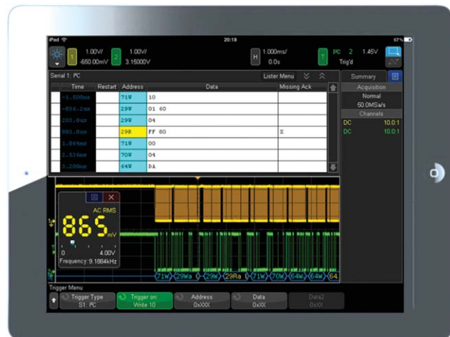
Figure 37: Tablet virtual front panel control.
