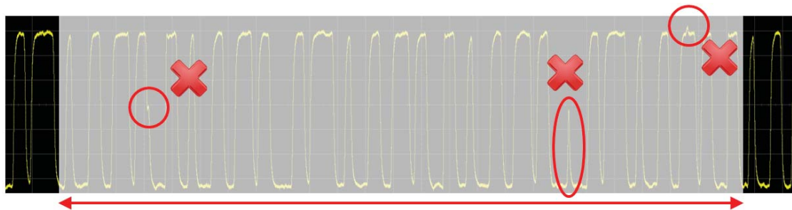
Figure 4: Other vendor's oscilloscope with 50,000 waveforms/second. A long dead time decreases your chances of capturing infrequent events.
