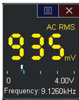
Figure 24: DVM 3-digit voltage and 5-digit frequency measurements always at your fingertips.
