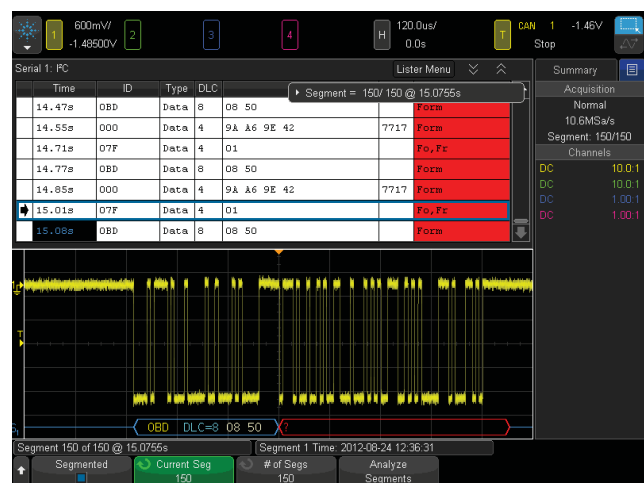
Figure 8: Segmented memory being used in conjunction with serial decode resulting in maximum insight into serial bus.
