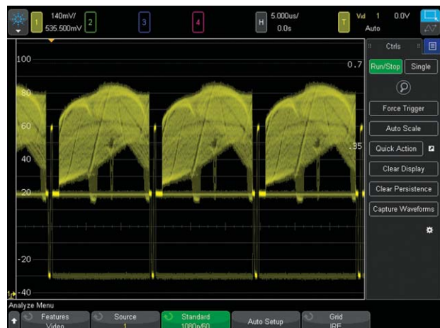
Figure 26: Triggering on 1080p HDTV signal analysis.
