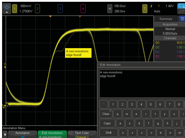
Figure 38(a): Annotation and keypad.
