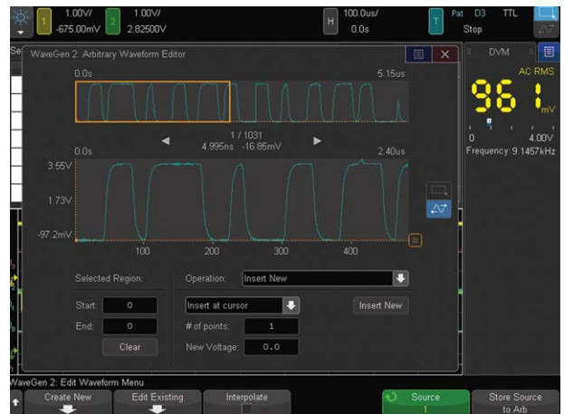
Figure 22: WaveGen arbitrary waveform editing screen.
