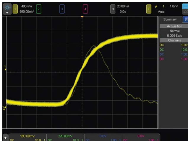
Figure 3: The 4000 X-Series captures a glitch occurring once in a million waveform cycles.
