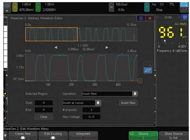
Figure 22: WaveGen arbitrary waveform editing screen.
