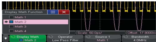
Figure 31: Four math functions can be created and nested with one resultant math function.
