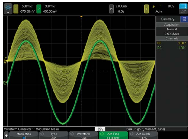
Figure 21: WaveGen sine wave output with and without added AM modulation.
