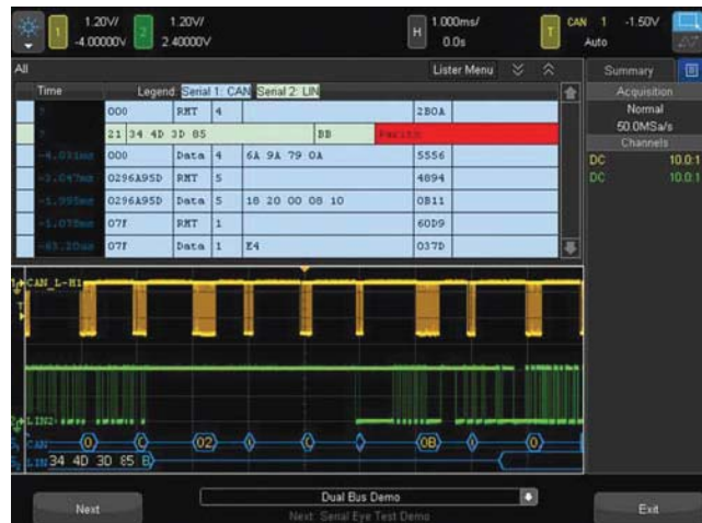
Figure 19: Dual serial bus CAN and LIN decode and interleaved “lister” display.
