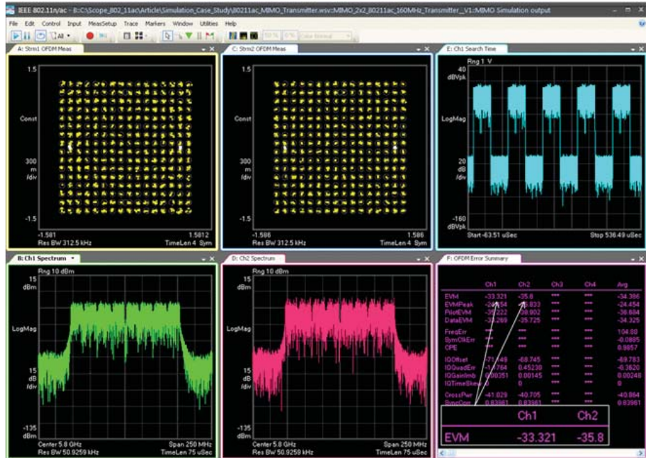
Agilent's 89601B Vector signal analysis software turns the 90000 Q-Series into spectrum analyzer
