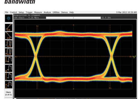
10 Gbps signal captured with 62 GHz of bandwidth, notice the faster rise time and wider eye measurements
