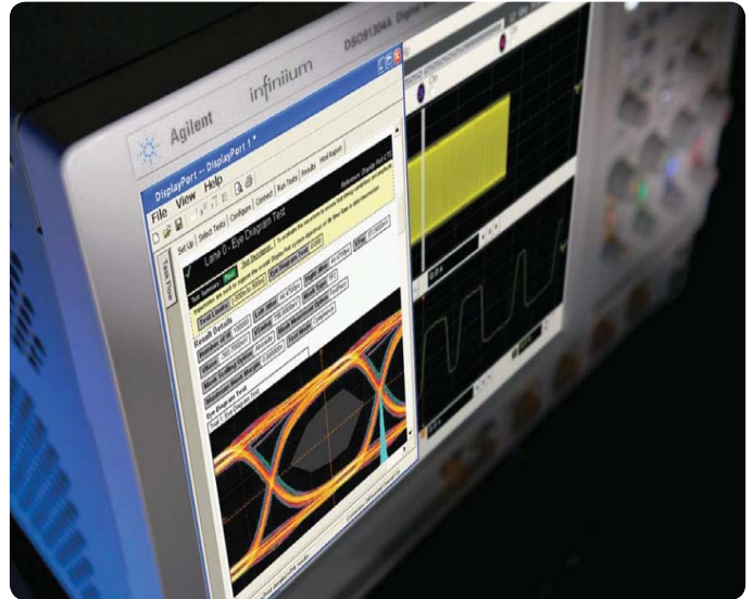
The DisplayPort electrical test software results report documents your test, indicates the pass/fail status, the test specification range, the measured values and the margin
