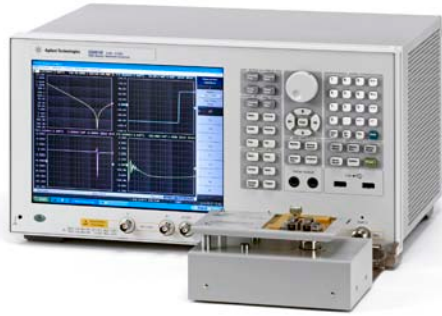
S-parameter port 1 reflection method
