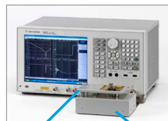
16092A fixture 16201A adapter Impedance measurement with reflection method (for 1 Ω to 2 kΩ) 1
