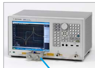
16047E fixture Impedance measurement with gain-phase series-thru method (for 3 Ω to 40 kΩ) 1
