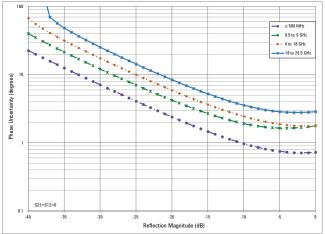
Power level of -15 dBm, 10 Hz IF bandwidth, no averaging, and 30-minute warm-up time. Includes uncertainties due to drift, noise, compression, and dynamic accuracy. Coverage factor of x1 applied to uncertainties, for ease of comparison with other industry handheld analyzers.
