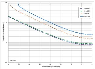
Power level of -15 dBm, 10 Hz IF bandwidth, no averaging, and 30-minute warm-up time. Includes uncertainties due to drift, noise, compression, and dynamic accuracy. Coverage factor of x1 applied to uncertainties, for ease of comparison with other industry handheld analyzers.
