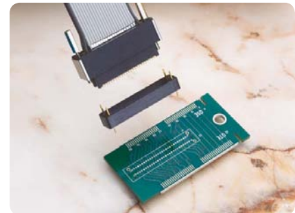
Soft touch connectorless probes reduce cost and shorten your design cycle by eliminating probing connectors
