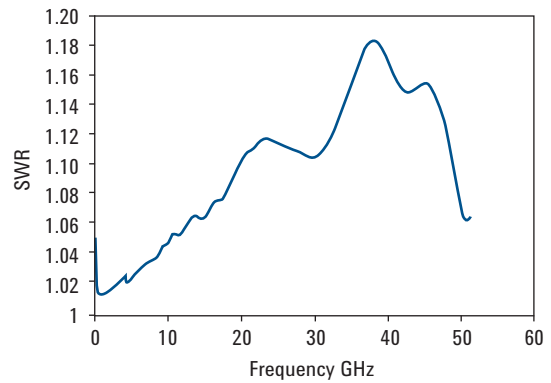
Typical SWR, 50 MHz to 50 GHz ( 25\text{ }^{\circ}\text{C} \pm 10\text{ }^{\circ}\text{C} ) for N8487A power sensor
