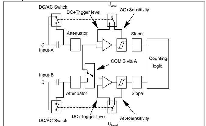
Figure 7 Input Circuit Block Diagram.
