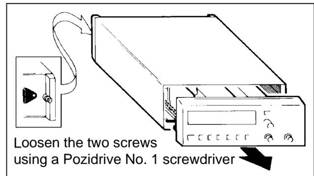
Figure 5 Loosen These Screws to Remove Cover.
