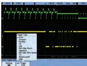
Trigger on and decode CAN serial packets.
