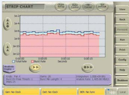
Bit error rate trends are easily seen on a Strip Chart. Thermal cycling or changing conditions that affect communications can be tracked.
