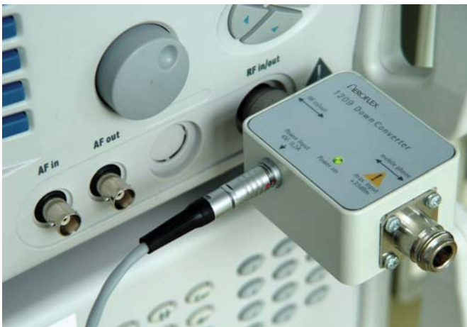
Figure 2: The 1209 Downconverter is an optional frequency extension for Bluetooth, WLAN, GPS tests and Mobile TV standards.
