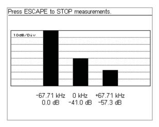
The large dynamic range of 60 dB for I/Q alignment allow for optimal tuning of phones. The bar graphs are clearly visible and the numbers provide accurate results.
