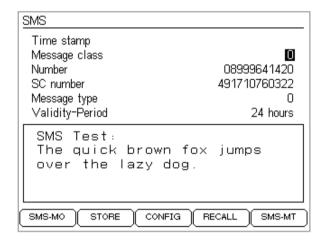
The SMS test capabilities of the 4202S offer analysis of the most crucial parameters used for SMS, such as Service Center Number, Validity Period and Message Class. This allows a service technician to pinpoint possible problems in the transfer of short messages.
