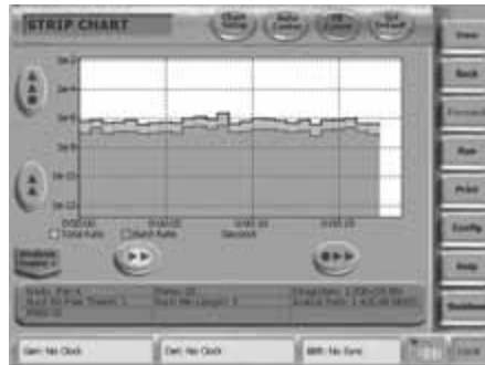
Viewing bit and burst error performance over time. This can be useful while temperature cycling as part of troubleshooting, for example.
