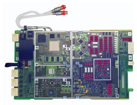
The Agilent 93000 14-Bit 100 MHz Digitizer provides true 14-Bit resolution for testing next generation set top boxes (STB), digital TVs (DTV) and Cable Modems.
