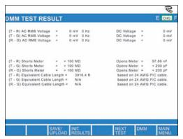
Measure AC/DC voltage, resistance and capacitance.
