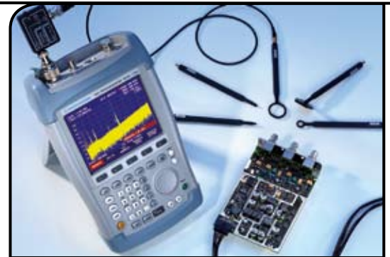
R&S®FSH with near-field probe set and DUT
