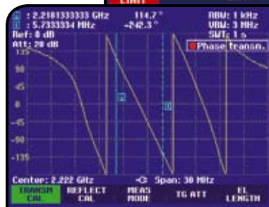
Measurement of phase
