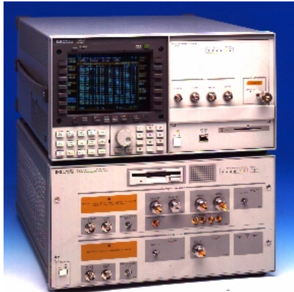
HP 71612B error performance analyzer available with pattern generator, error detector and integral 12 GHz clock source.
