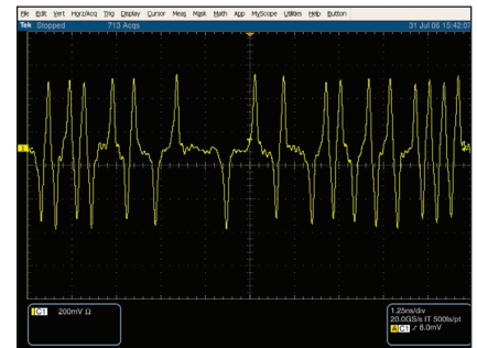
Figure 4: Hard disk read channel signal (5 Gb/s 2 points per cell); AWG7121B with 10 GS/s.
