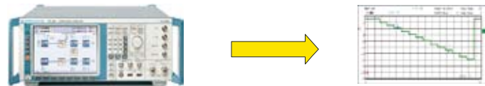
The R&S®SMU200A changes the code channel output power on the basis of the TPC field
