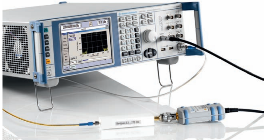
Scalar network analysis on an external bandpass filter (with R&S®SMF-K28 power analysis option plus R&S®NRP-Zx power sensor)
