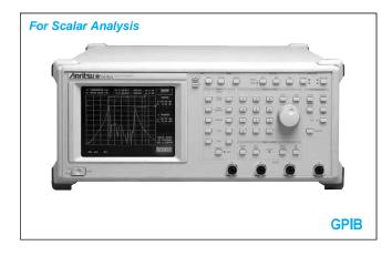
The 56100A Scalar Network Analyzer measures insertion loss, insertion gain, or RF power with 76 dB dynamic range. Measure device match as return loss in dB or as SWR. Separate detectors can be used on all four inputs for multiple transmission measurements on duplexers or matched amplifiers.
