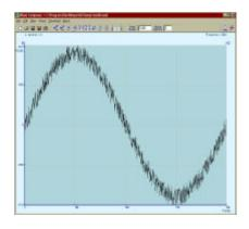
The above waveform was created using simple elements that are built into the Wave Composer. The waveform is a sine with an added second harmonic and topped with random noise. Downloading this waveform to the 3155 is done in a few milliseconds
