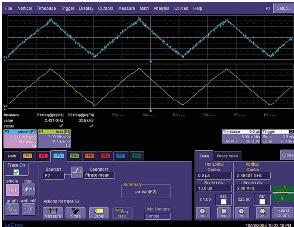
See multiple cycles of spread spectrum clocking.
