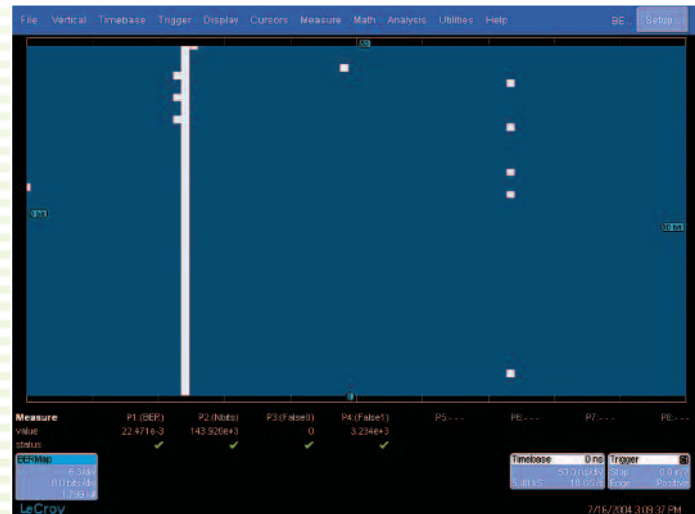
The bit error map displays the location of bit errors (shown as bright squares) relative to their location in a frame or pattern. Each frame is displayed as a row in the plot. Frames can be of fixed length, delimited by a specific bit pattern, or both. The bit error rate, along with the number of bit errors, is displayed below the map.
