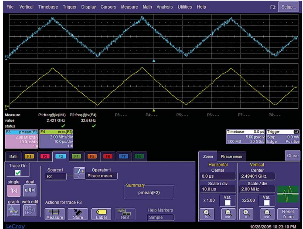
See multiple cycles of spread spectrum clocking.
