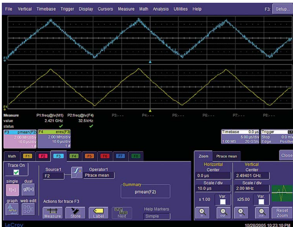
See multiple cycles of spread spectrum clocking.
