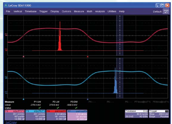
SATA compliance test maximum voltage check.
