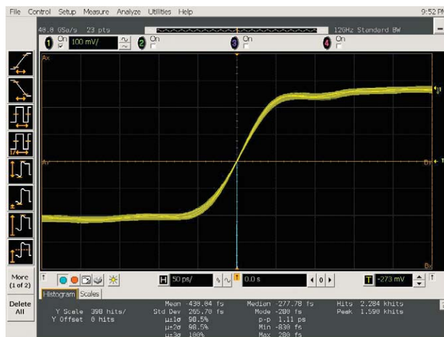
Figure 8. With the industry's lowest trigger jitter – less than 500 fs rms (typically, less than 200 fs rms on 5 Gb/s PRBS signal) – the DSA80000B facilitates accurate waveform viewing of multiple waveforms.
