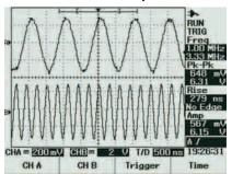
CH1 and CH2 waveforms, along with the Dual channel Math waveform, trigger levels, horizontal positions, offsets, V/div and Time/division settings are displayed.
